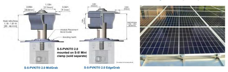
The S-5-PVKIT® 2.0 is mounted with the S-5!® Mini clamps suitable for the respective standing seam. The stainless steel module support disc of the S-5-PVKIT® 2.0 has optimized teeth which enable the grounding of the modules. Therefore, no straps or wires are required, except for connecting one module column to another and grounding the complete system (UL 2703 Listed).
